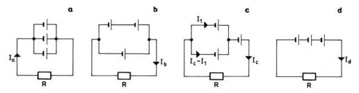
The other possible ways of connecting the cells involve different polarization of the cells, and are thus less favourable.
