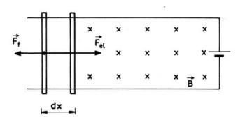
The motion of the rod is determined by a force  $\vec{F}$  which is the resultant of two forces: the electromagnetic force  $\vec{F}_{el}$  and the force of friction  $\vec{F}_f$ .
