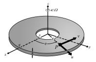
The polar coordinates r and φ of the position of rest P of a vibrating particle in the annular disc of density ρ, height h, rotating slowly at rate εΩ. The vibrating particle at P has radial displacement u and tangential displacement v
