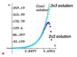
• The accuracy of the routine can be gauged by observing the difference (estimated error) between the numerical solutions.
