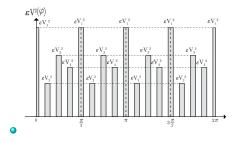
• Because of the periodicity involved with the potentials, we may determine a Fourier series for the function  $V^2(\varphi)$  depicted in the figure as follows
