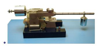
• A small amount of explosive is spread onto the rough surface of the tile and a blunt pin is dragged across the rough surface. The amount of force needed to ignite the explosive can be varied as illustrated above.
