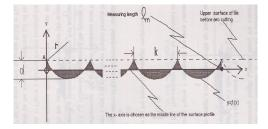
• The arithmetic mean roughness value (ISO/DIS 4768/1) of a surface is defined as
