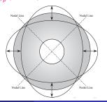
• When m = 2 the vibration pattern has four nodes:
