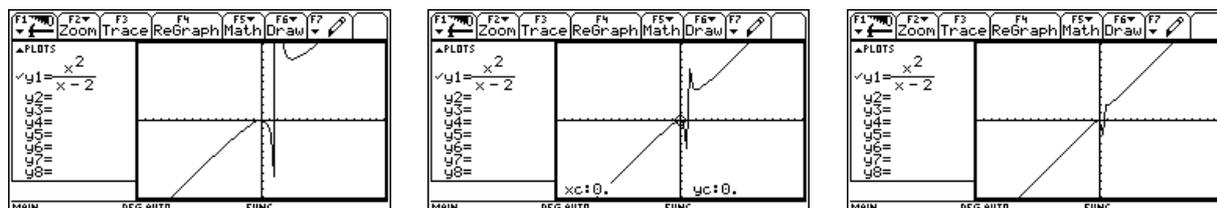
Now we have to find a suited linear function fitting well to the rational function. By inspection of the graph we suggest that the slope of the linear function should be  $k = 1$ . Our first guess is  $y_2(x) = x$ .
