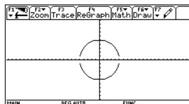
The second method was to plot the circle as a parametric function. Therefore we have to define parametric functions for the x-coordinates and for the y-coordinates of the points lying on the circle. The parameter must be called  $t$ . If we choose appropriate settings for the window we obtain the image of a circle without holes.
