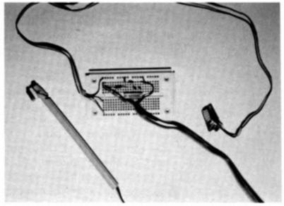
The entire light pen system, comprised of the breadboard, the ink-pen-based light pen, and the 9-pin connector, can be used for a multitude of programming applications, from drawing programs to menu selection.
